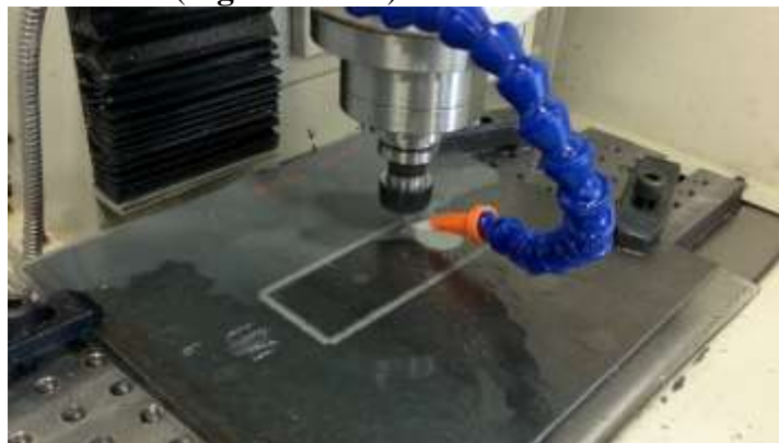
Figure 4-2: Manufacturing of the main frame using the Tormach CNC mill
