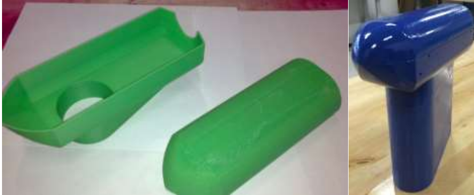
Figure 4-5: Prototyped nacelle (Left); Finished and painted nacelle (Right)
