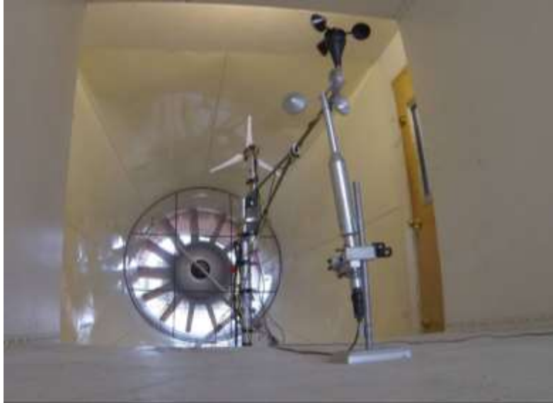
Figure 5-1: Wind tunnel used for wind turbine testing
